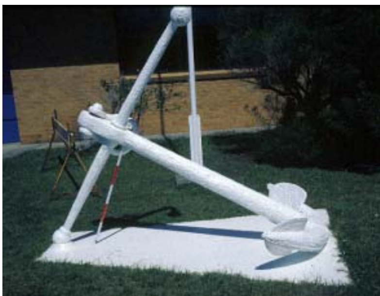
Figure 7: An Admiralty Pattern anchor on display at the Coffs Harbour Water Police office. Photo: David Nutley.
